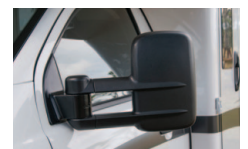
Clearview extendable and foldable power mirrors are standard on Navigator and an option on Compass
